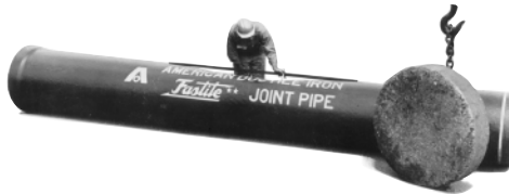
After receiving the full force of a 2-ton weight dropped from a height of 9m, this 800mm ACIPCO Ductile Iron pipe was severely deformed, but did not fail.
